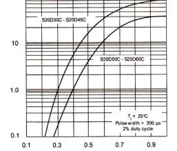
VF, INSTANTANEOUS FORWARD VOLTAGE(V) Fig-2 Typical Forward Voltage date per Element.
